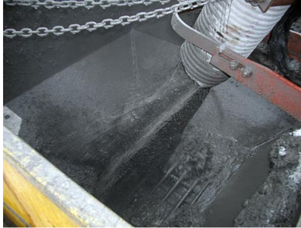
Figure 7 – Example of underground mine backfilling with tailings, at Cleveland Potash, Boulby Mine, UK. (Source: Tailings.info, 2012)
